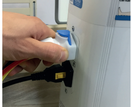
4. Connect the Sixtube connector to the controller with the blue release button facing up and make sure the connector snaps when locking into place.
