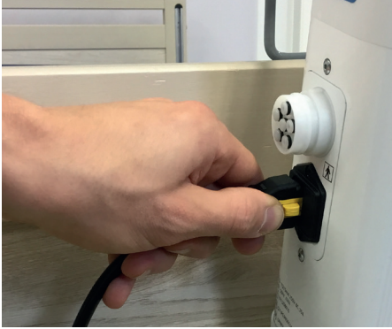
3. Connect the power cable to the mains connector of the controller.
